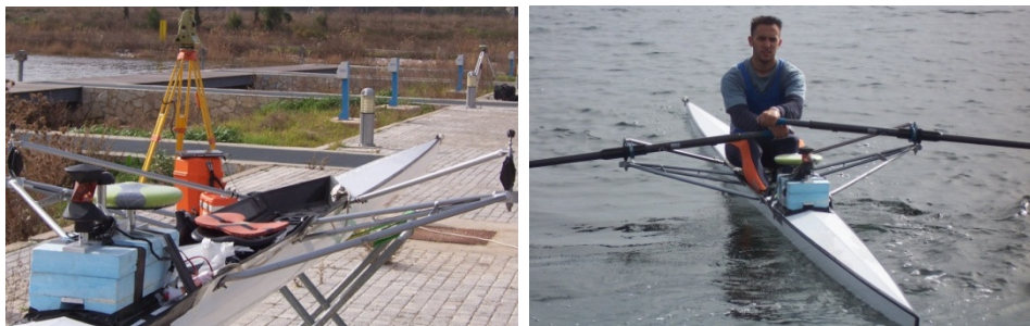
Fig. 4. GPS and MEMS-IMU configuration used during preliminary testing at Shinias Olympic Rowing and Canoeing Center
